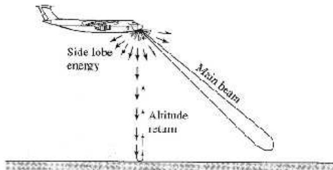
**Fig. 4.9** Sketch of airborne Pulse Doppler radar
