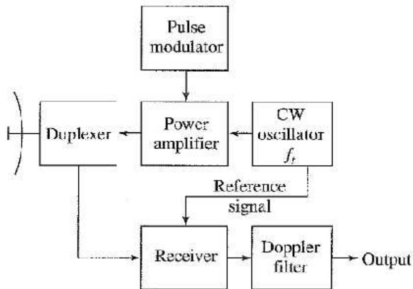
**Fig. 4.4** Block diagram of simple Pulse Radar
