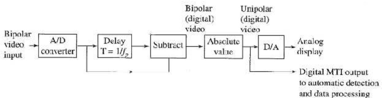
Fig. 4.6 Block diagram of single delay line canceller
