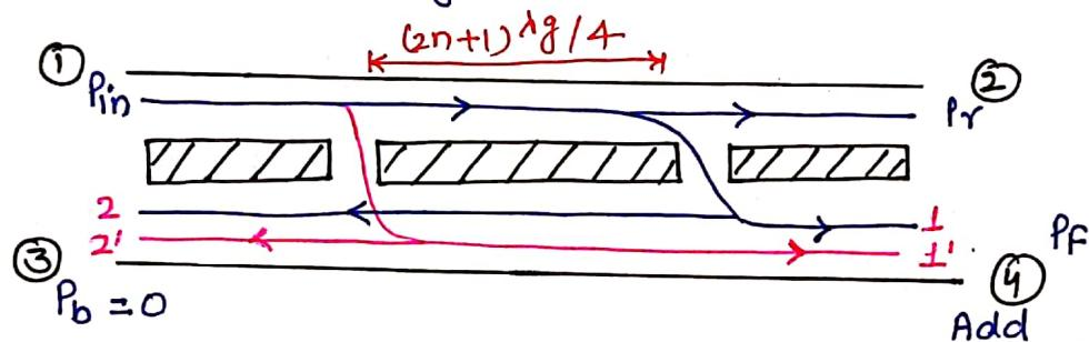
→ Gap between two holes should be odd multiple of  $\lambda g/4$  so, that the power at port ④ get added and power at port ③ will cancel out each other.
